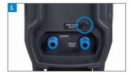
**Step 4.** Attach the pump hose to the water inlet on the front of the appliance. To attach pull back the collar of the quick connect fitting and push on the water inlet firmly, once connected ensure the collar is pushed forward to lock it in place.
