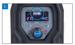
**Step 3.** Connect to the DC input socket (red) at the rear of the appliance. The battery charge level will start to flash and move from red to green confirming that the battery is now charging.
