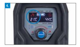
**Step 5.** Taking care to measure the temperature of the water from the shower head, the temperature can be adjusted by turning the gas control until the desired level is reached.
