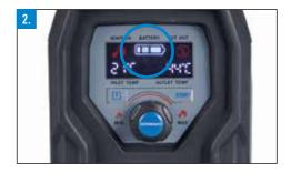
**Step 3.** Position the gas temperature control in the central position between MIN and MAX. Then press the START button and water will start to flow within a few moments.
