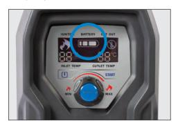
**Step 3.** Connect to the DC input socket (red) at the rear of the appliance and the battery charge level will start to flash and move from red to green confirming that the battery is now charging.
