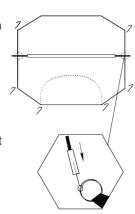
To make sure the tent stays in place, insert the pegs into the ground at a 45° angle.
